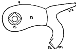
Fig. 35. Hammer, half size. a , body; b , head; c , comb; d , countersink, slit, and knife-edge; e , pivot-hole.
